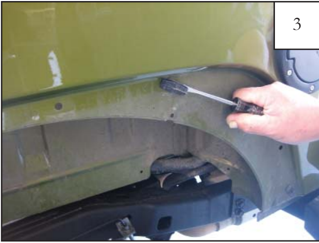
Using a pry tool or flat head screwdriver, remove any plastic clips still in fender.
