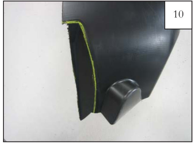
After trimming, mark the rear portion of the splash shield as shown and trim. NOTE: If trimmed too little, flare won't fit; if trimmed too much, shield won't stay behind flare.
