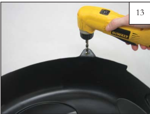
Use a drill and 5/16" drill bit to drill through mark made on rear mounting tab.
