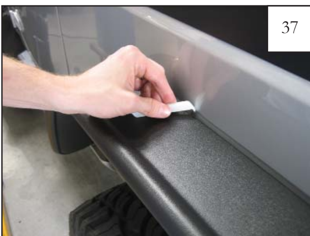
Use the hooked end of the edge trim tool to check for full adhesion. Do this by sliding it along the top of the edge trim to visually verify that the tape is adhered to the vehicle surface. Repeat step 36 if the tape is not fully adhered to the vehicle surface.
